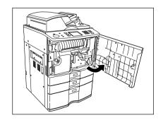
2 Rotate the left end of the holder, then pull out the empty toner bottle with both hands as shown on the right.
